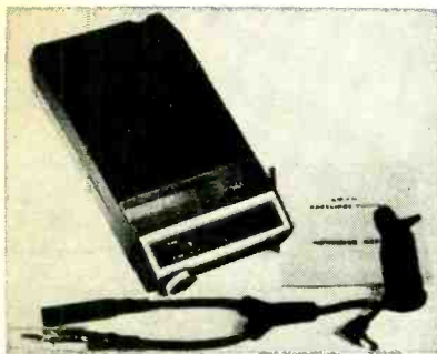
CARTRIDGE TUNERS plug into cartridge tape players and convert them into FM or AM/FM radios. GC's 30-3075 shown.
