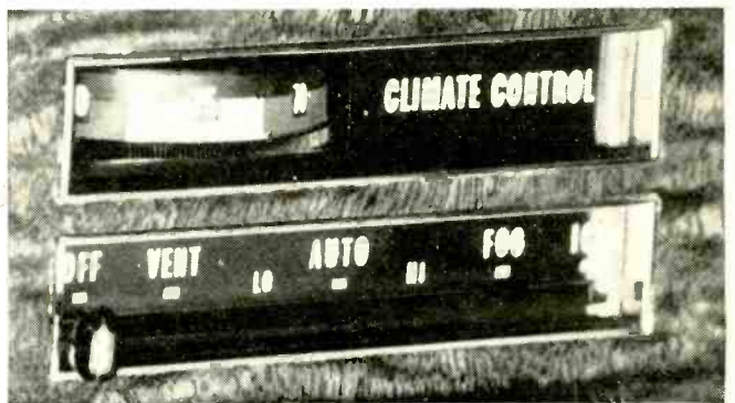
FOUR-SEASON CLIMATE CONTROL is directed by electronic sensors. Thermistors read internal temperatures and direct switching and blending of heater and air-conditioner outputs.
