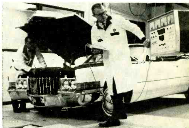
DIAGNOSTIC CONSOLE feeds car performance characteristics into a computer at this Cadillac center in Brooklyn, N. Y. The computer compares operation with preset specifications and prints out a complete report. New BMW cars rolling off the line include built-in transducers connected to a jack positioned under the hood. Drive into a diagnostic center, plug in the tester and minutes later you find out how well your car is performing.
